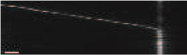
**Figure A9:** Determining the processivity of kinesin-1 motors. Typical example of a kymograph obtained from stepping motility assays using single kinesin-1 molecules attached to quantum dots, under the same experimental conditions (salt, ATP, oxygen scavenger etc.) as used in the doublet experiments. Bar, 1  $\mu\text{m}$ . Total time: 40 s.
